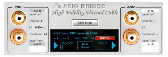
If there is an ASIO Clock problem, the measured sample rate (here 44100 Hz) is shown in a blinking red rectangle.
