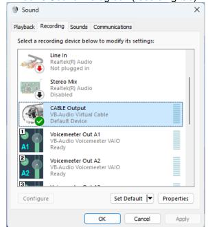
VB-CABLE for Win10/11 x64/Arm64 installs 2x different inputs. The first is a speaker playback device (that can be setup with configure button) limited to 8 channel (7.1 speaker config). The Second CABLE input is a Line Out pin able to manage up to 16 channels. Both are setup in stereo 48kHz by default.
