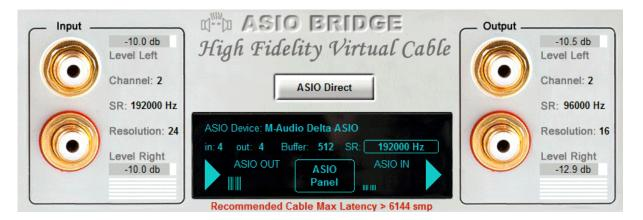
The red text below the LCD is displayed when current Cable Latency is too small to support current audio stream.
