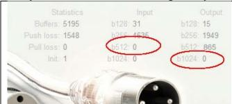
Here, according statistics, the stream of the Audio Source Application is using 512 sample max buffer while the stream of the Audio Recorder application uses 1024 samples Max Buffer.
