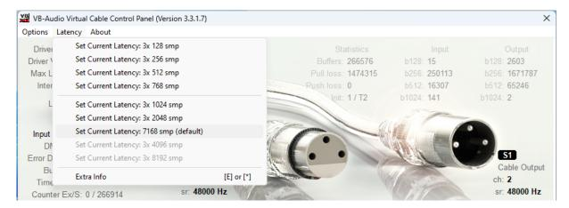
If the latency is considered too small according statistics (buffer used by applications connected to the cable) the counter becomes red and the sound can become discontinued or simply silence.
