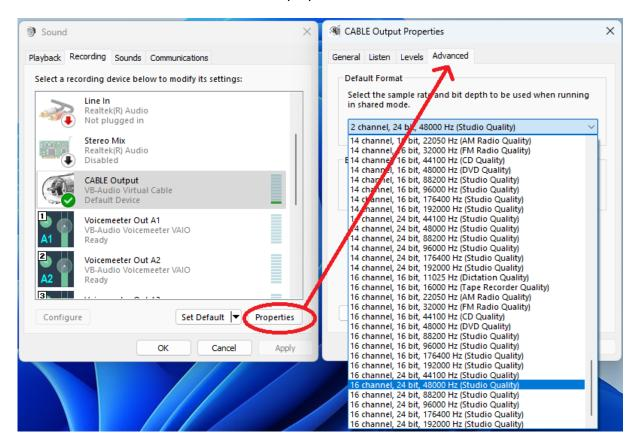
VB-CABLE previous version (XP to Win7) is limited to 8 channels. The 8 channels are also present on VB-CABLE output (recording device) but can be used with MME under XP only. MME is limited to stereo from Vista. But the 8 channels are available though KS interface. WIN10/11 version provides 8 channels (or up to 16) for all interface (MME, WASAPI, KS).
