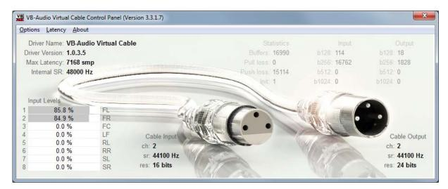
The VB-CABLE works internally with a fixed sample rate and a fixed pipe size (7168 samples per default) and support I/O sample rate range from 8kHz to 96 kHz.
